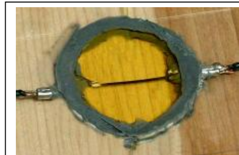
Photograph #1: MicroCell Used to Test Oils for Film-Forming Compounds
