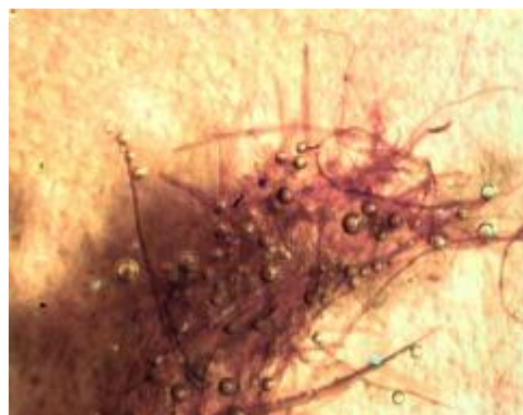
Photograph #2: Gas Released by Sulfites in Paper Insulation
